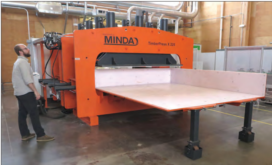
A TimberPress X 225, made by Minda Industrieanlagen GmbH, a German company, will allow researchers at Oregon State University's Advanced Wood Products Laboratory to produce cross-laminated timbers for testing. The press can handle CLT panels up to 18 feet long, eight feet wide, and six inches thick. Photo by Steve Wilent.
