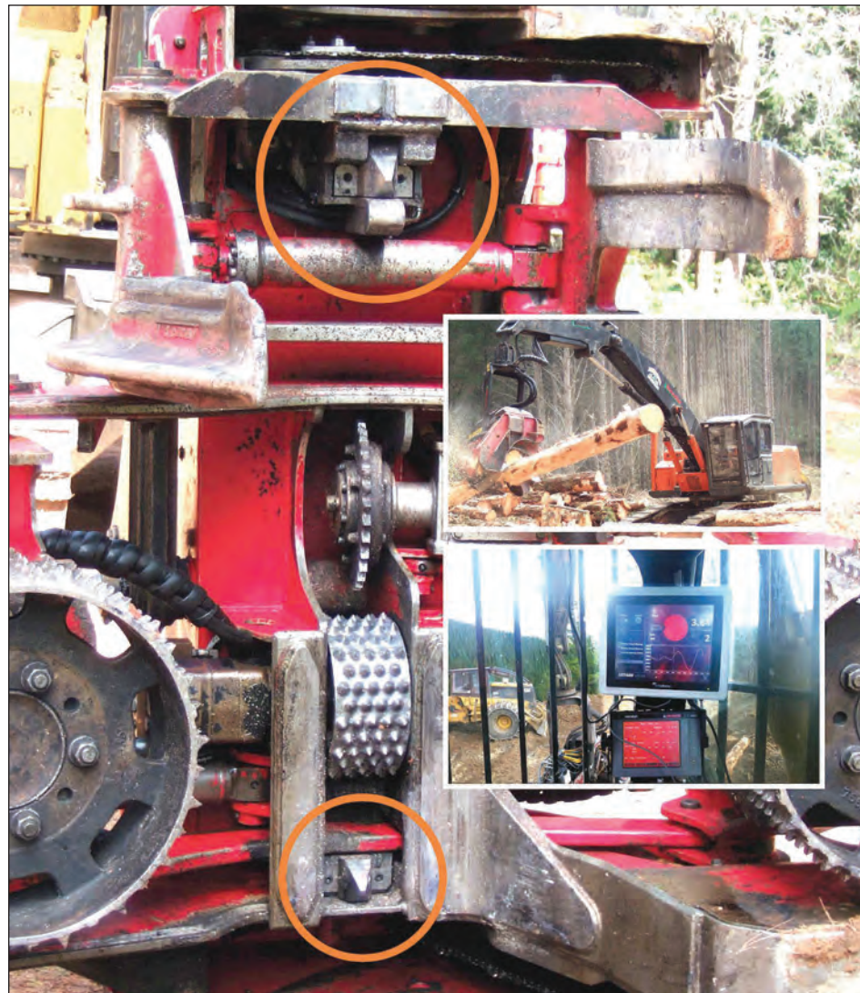
Fibre-Gen's Hitman PH330 is an automated, real-time wood-quality measurement tool that can be mounted on harvester processor heads. Data from the sensors (circled) are displayed on a screen in the cab, allowing the operator to sort logs for hauling to the appropriate destination. The New Zealand-based company makes several other tools for measuring wood quality. For more information, see fibre-gen.com .
