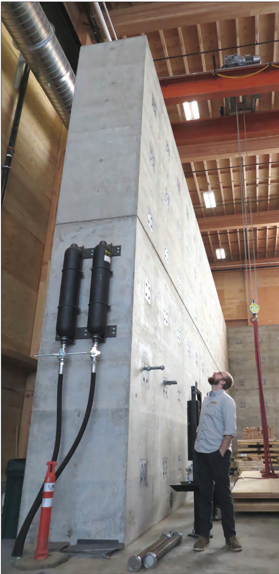
The Advanced Wood Products Laboratory includes a structural testing bay with a 25-foot-tall, four-foot-thick strong, or reaction, wall for anchoring model buildings up to three stories high during structural tests. The bay features a reinforced concrete floor 60 feet wide, 80 feet long, and five feet thick. This is one of the largest strong wall/floor systems for wood-products research in the US. Photo by Steve Wilent.
