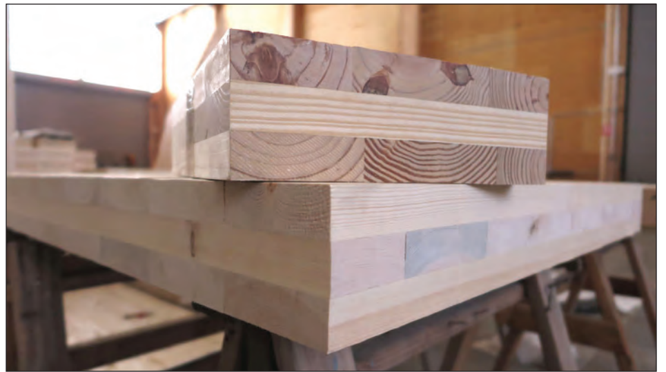
Two cross-laminated timber sections: one made of southern yellow pine (top) and the other of spruce-pine-fir lumber. Photo by Steve Wilent.
