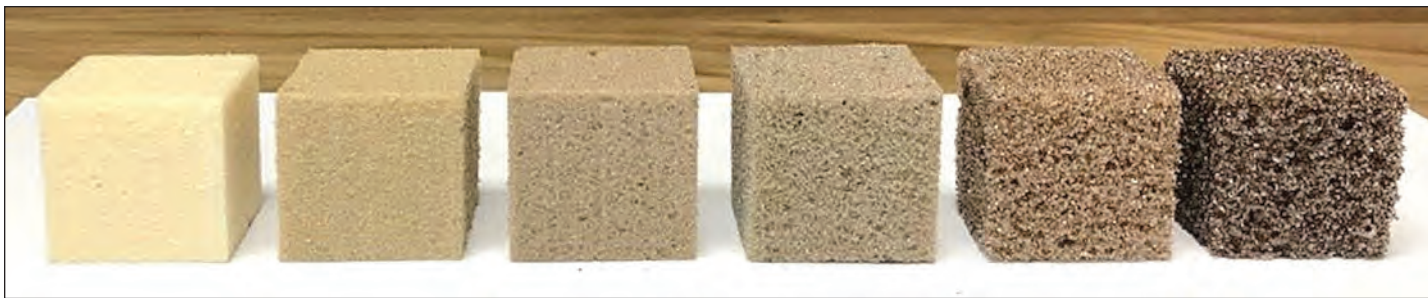
Examples of rigid foam created at Michigan State University that run the gamut of zero to 100 percent lignin content.
