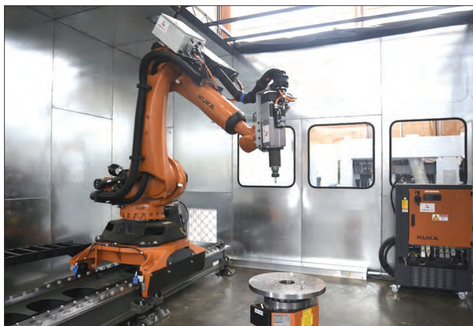
A six-axis robotic arm made by Kuka AG, a German company, will cut holes and channels for hardware in mass-timber panels for testing by researchers. Image: OSU.
