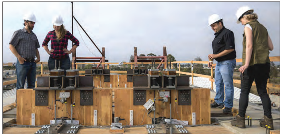
Researchers atop a two-story CLT structure that uses post-tensioned rocking shear walls as its lateral force resisting system. The structure rests on a "shake table" designed to simulate an earthquake. The researchers are examining load cells, sensors that measure tension in the steel rods inside the CLTs. The tests were completed in San Diego in 2017 as part of a multi-institutional collaboration funded by the National Science Foundation's Natural Hazards Engineering Research Infrastructure unit. The researchers will make similar tests of a 10-story timber structure in 2021 as part of continuing research into the seismic performance of timber buildings. Photo: Erik Jepsen.
