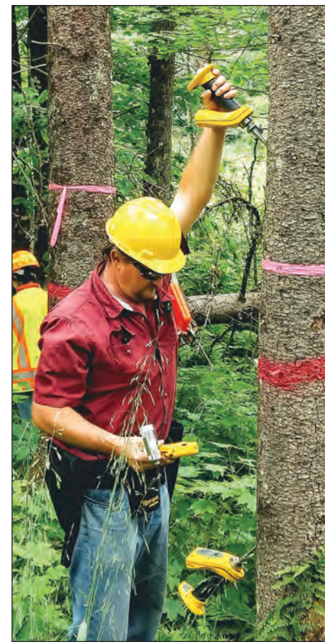
Researchers test devices that test the quality of the wood in standing trees using acoustic velocity measurements that gauge wood stiffness. Image courtesy of Robert Ross.
